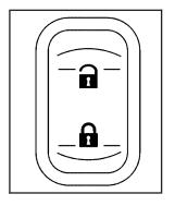
A power door lock switch is located on both front doors next to the door handle.
